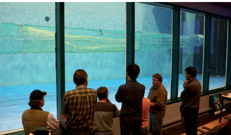
Testing a salmon excluder net in a flume tank. John Gruver et. al. St. John's, Newfoundland.
