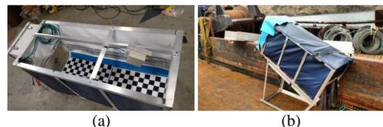
Fig. 1. Chute with a static camera, a) interior view with checkboard for calibration, b) installation with cover on board.
