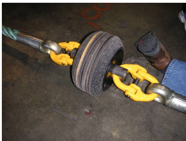
10 inch elevating bobbin connected to 2 inch (52mm) combination wire with hammerlocks (coupling links)
