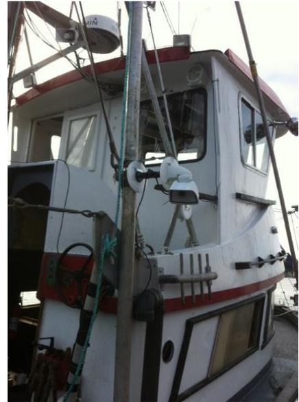
**Figure 2. Typical rail mounting position for a scientific data collection camera.**
