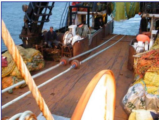
Setting sweeps and bobbins off the forward net reel
