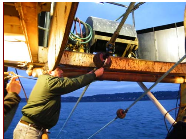
Measuring bobbin clearance off the aft net reel
